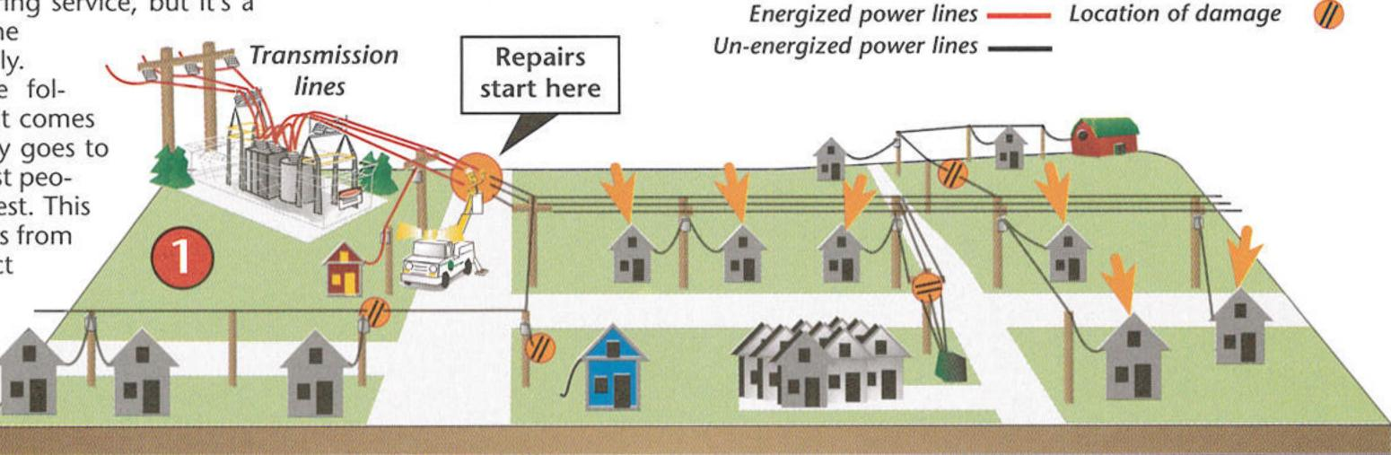
Step 1: The substation is energized but a main distribution line is damaged near the substation, leaving most members without power.
